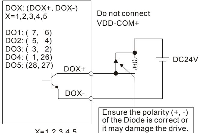
Use a relay or open-collector transistor to input signal.
