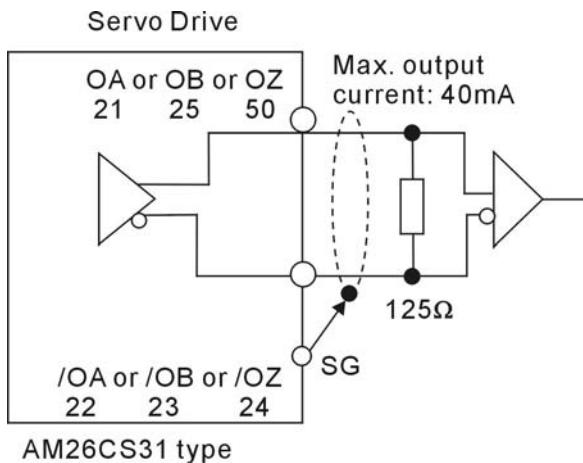
**C12:** Encoder output signal (Photocoupler)
