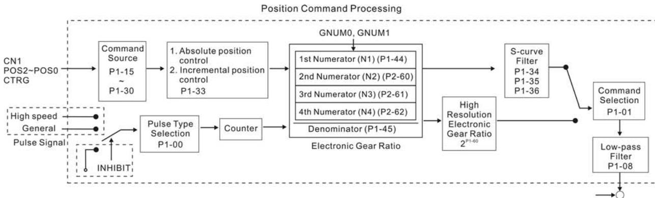
Using parameter can select Pr mode and Pt mode. Electronic gear ratio can be set in both two modes to set proper position revolution. ASDA-A and ASDA-A+ series servo drives also provide S-curve and low-pass filter, which are used whenever the motor and load need to be operated more smoothly. As for the information of electronic gear ratio, S-curve and low-pass filter, please refer to the following sections 6.2.4, 6.2.5 and 6.2.6.
