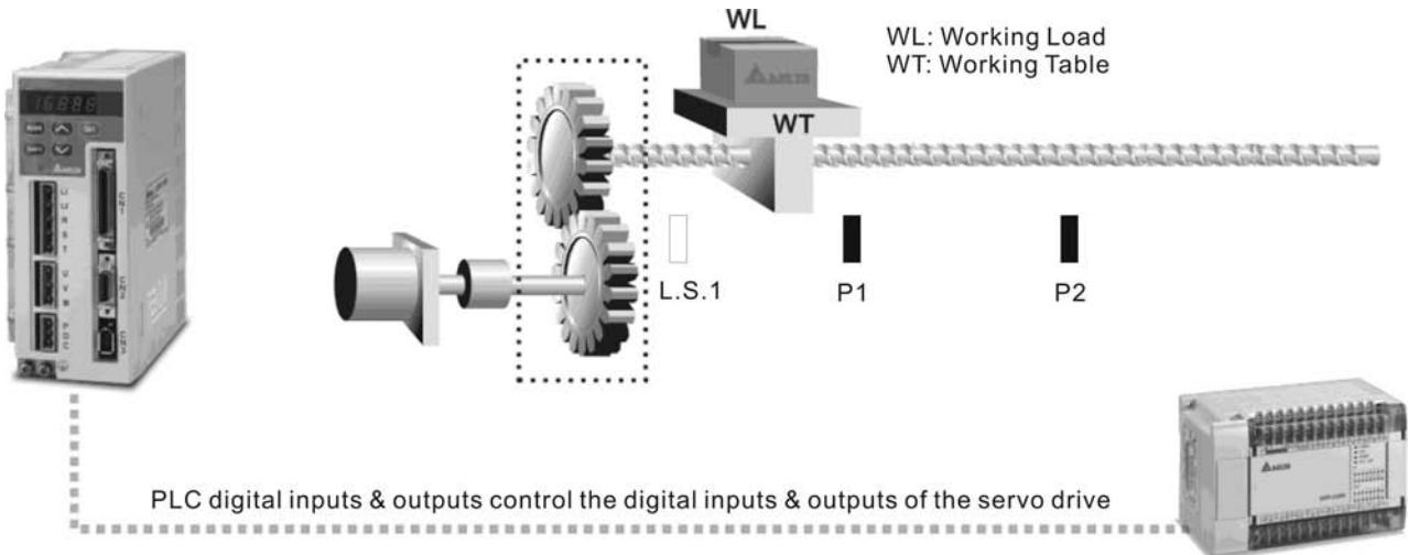
Suppose that the machine will move to limit switch (CCWL), L.S.1 when motor is in forward rotation (from motor shaft view) and the machine will move to limit switch (CWL), L.S.2 when motor is in reverse rotation, if limit switch is set, L.S.1 as "Home", the machine will be positioned between P1 and P2 according to working procedure.
