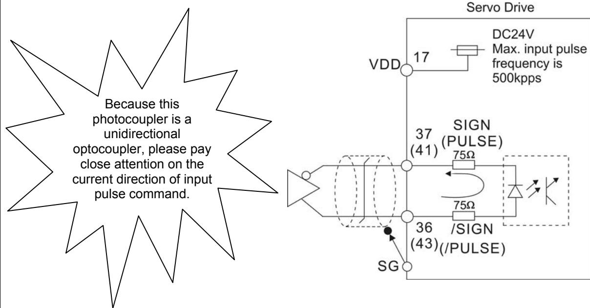
**C4-2:** High-speed pulse input (Line driver)
