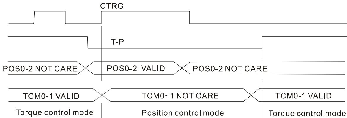
Figure 3. : Torque / Position Control Mode Selection
