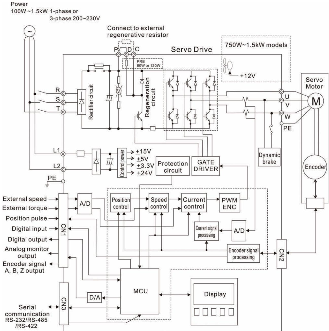
Figure 3.6 Basic Wiring Schematic of 2kW ~ 3kW models
