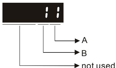
A: Decimal place setting of internal speed command.
