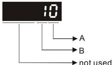
A: Monitor analog output polarity
