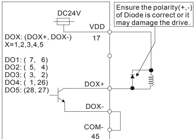
**C7:** Wiring of DO signal, for the use of external power supply, general load
