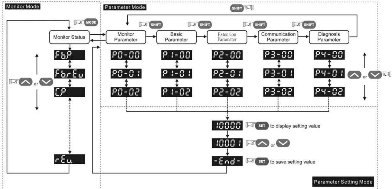
1. When the power is applied to the AC servo drive, the LCD display will show the monitor function codes for approximately one second, then enter into the monitor mode.
