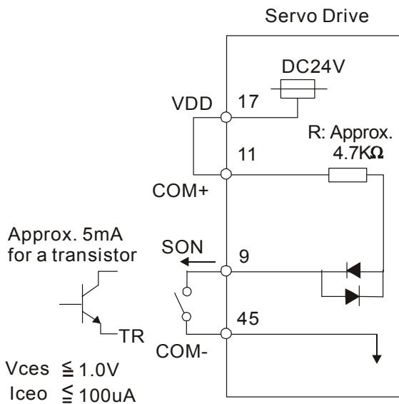
**C10:** Wiring of DI signal, for the use of external power supply
