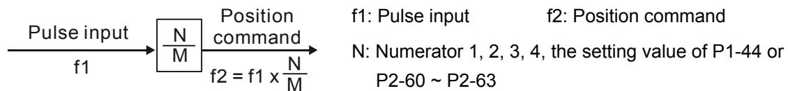
The electronic gear ratio setting range must be within:  $1/50 < N/M < 200$ .
