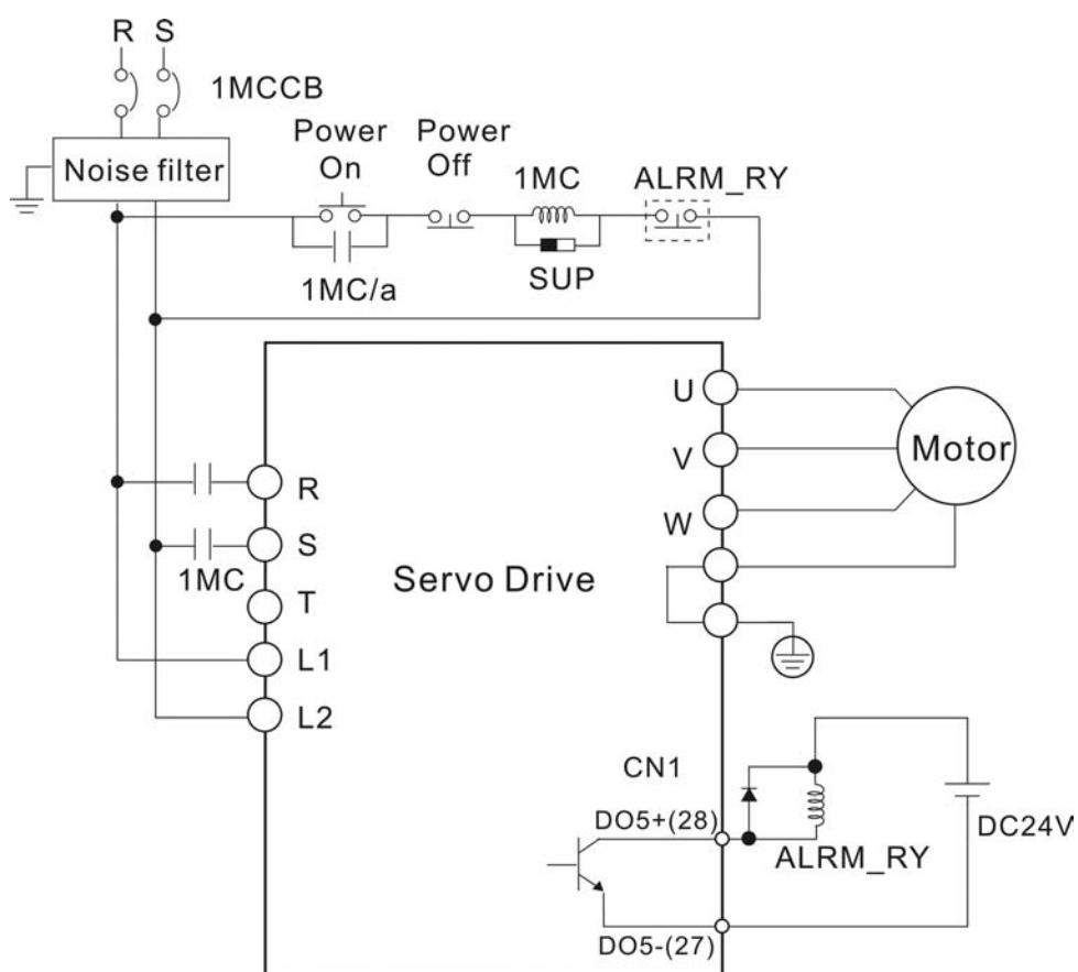
**Figure 3.3 Three-Phase Power Supply Connection**
