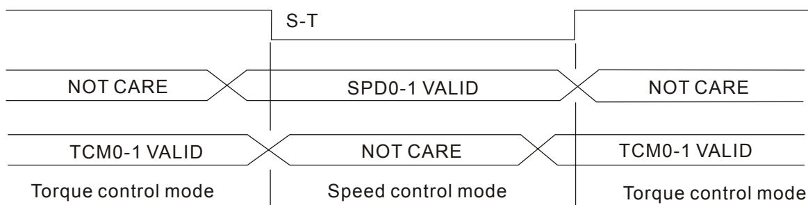
Figure 2. : Speed / Torque Control Mode Selection
