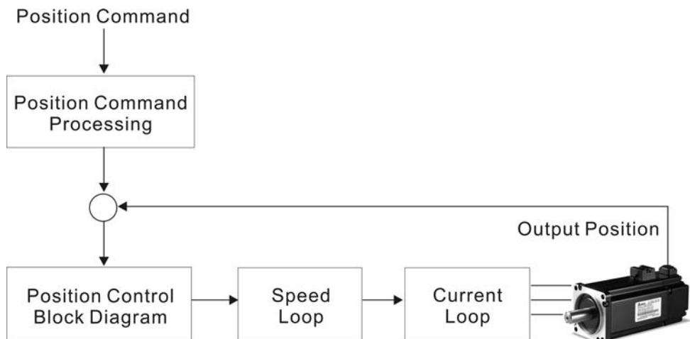
In order to pursue the goal of perfection in position control, the pulse signal should be modified through position command processing and the structure is shown as the figure below:
