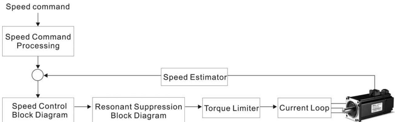
In the figure above, the speed command processing is used to select the command source of speed control according to chapter 6.3.1, including proportional gain (P1-40) and S-curve filter smoothing strategy of speed control. The speed control block diagram is used to manage the gain parameters of the servo drive and calculate the current input provided to motor instantaneously. The resonance suppression block diagram is used to suppress the resonance of mechanical system.
