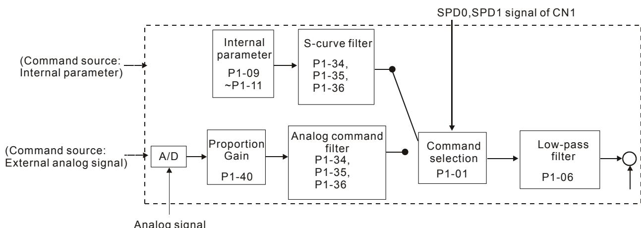
The command source is selected according to the state of SPD0, SPD1 and parameter P1-01 (S or Sz).
