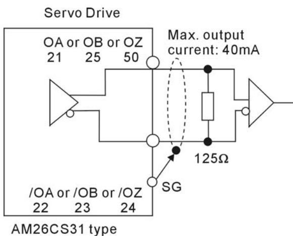
**C12:** Encoder output signal (Photocoupler)
