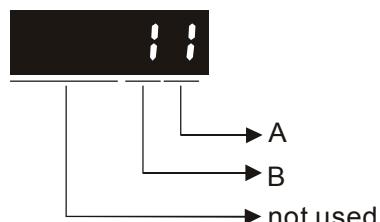
Value A: decimal place setting of internal speed command.
