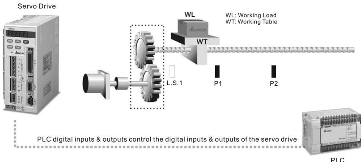
Suppose that the machine will move to limit switch (CCWL), L.S.1 when motor is in forward rotation (from motor shaft view) and the machine will move to limit switch (CWL), L.S.2 when motor is in reverse rotation, if limit switch is set, L.S.1 as "Home", the machine will be positioned between P1 and P2 according to working procedure.
