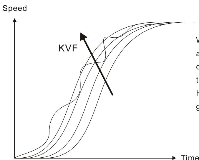
When the value of KVF is nearly to 1 and the forward compensation is more complete, then the value of dynamic tracking error will become very small. However, when the value of KVF is too great, it may cause vibration.
