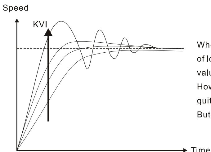
When the value of KVI is greater, the value of low-frequency gain is also greater and the value of steady error is nearly zero (0). However, the value of phase margin will reduce quite substantially. It is helpful to steady error. But it is not helpful to dynamic tracking error.
