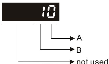
A: Monitor analog output polarity
