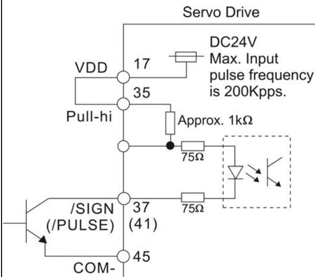
**C3-2:** Pulse input, for the use of external power supply (Open-collector input)
