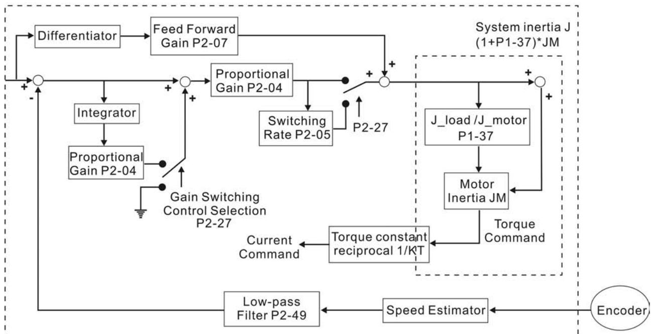
There are two turning modes of gain adjustment: Manual and Auto modes. The gain of ASDA-AB series servo drives can be adjusted by using any one of three tuning modes.
