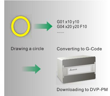
The graphic is converted into G-Code and further downloaded to DVP-PM before being drawn.
