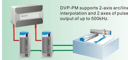
DVP-PM supports 2-axis arc/linear interpolation and 2 axes of pulse output of up to 500kHz.
