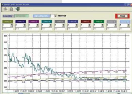
Through RS-458 interface, it is able to monitor 10 temperature controllers in one PC. DTCCOM provides graphic function to record temperature curve and the recorded data can be saved for future review.
